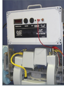
Field test unit and redundant sensing and firing logic
